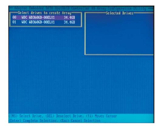
5. Press **Enter** when both disks for the new array are selected. The Array Properties menu displays (as the shown on the screen on the next page).
